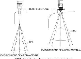
FIGURE 1 Rod and horn style radar detectors
