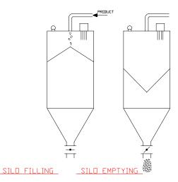
Drawing No 1. Ultrasonic level detector in a silo.
