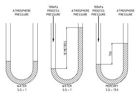
Figure No. 1 U-tube Manometers with Water and Mercury
